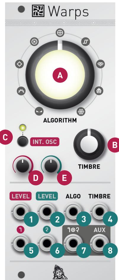
**D. External carrier amplitude** or **internal oscillator frequency.** When the internal oscillator is switched off, this knob controls the amplitude of the carrier, or the amount of amplitude modulation from the channel 1 **LEVEL CV** input (1). When the internal oscillator is active, this knob controls its frequency.
