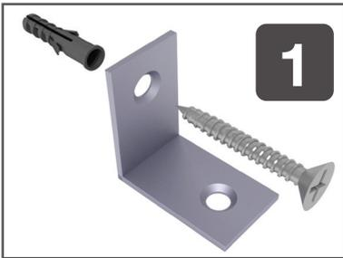
Using suitable screws and wall plugs, fix 2 L Brackets to the wall at the correct height to support the bottom edge of your tile. They should be located approximately 20mm in from the corners of the tile.
