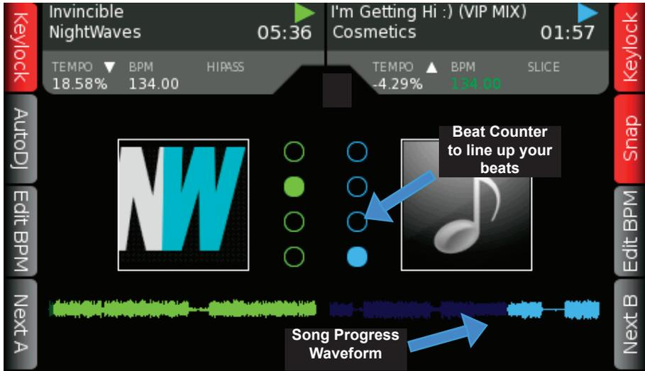
The **HOME/WAVEFORM** button, located below the LCD screen, is used to toggle between the **HOME** and **WAVEFORM** screens.
