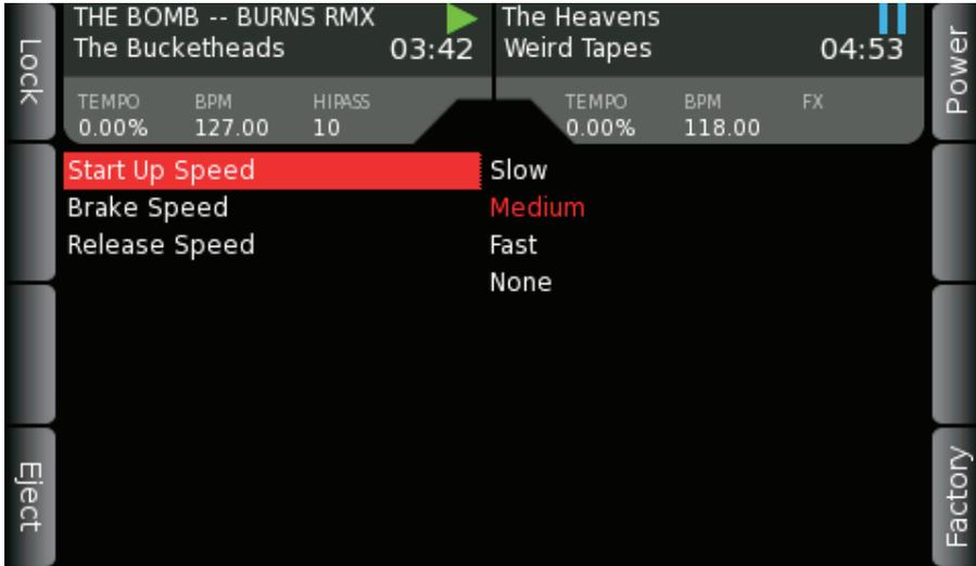
**Start Up Speed** – slow, medium, fast, none, the time it takes audio to ramp up to full speed when the Play button is pressed
