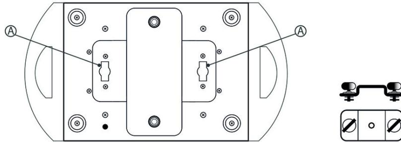
A Mounting points for 1/4-turn fasteners used for omega brackets
