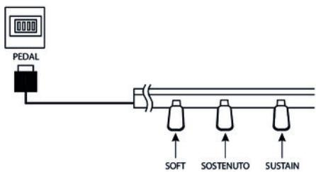
1. Connect the foot pedal to the provided connector on the bottom of the pedal box.
