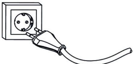
3. ➤ Plug the power cord into a 230 V AC outlet.
