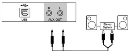
You can connect powered speakers, your stereo system or other amplifiers to the rear AUX output.
