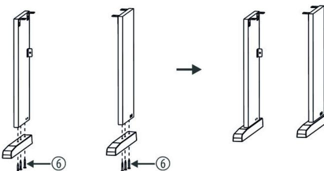
3. ➤ Screw the body feet to the side panels (6 x screws 6 x 60).
