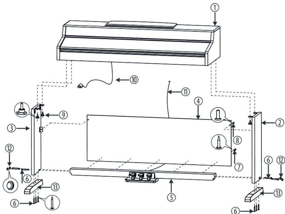
You need a Phillips screwdriver (not supplied) for the assembly of the digital piano. Open the package and please make sure before assembling that the entire scope of delivery is present, as posted here.
