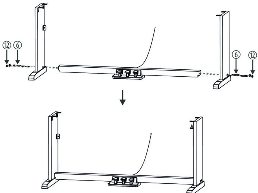
4. ➤ Screw the pedal box to the two side panels (4 x screws 6 x 60) and insert the four supplied plastic caps into the screw holes.
