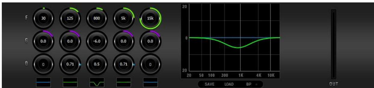
Antelope Audio's integrated **EQ** offers 5 fully parametric bands, two of those can work in filter or shelving mode and the three in the middle can cut or boost selected frequency ranges.
