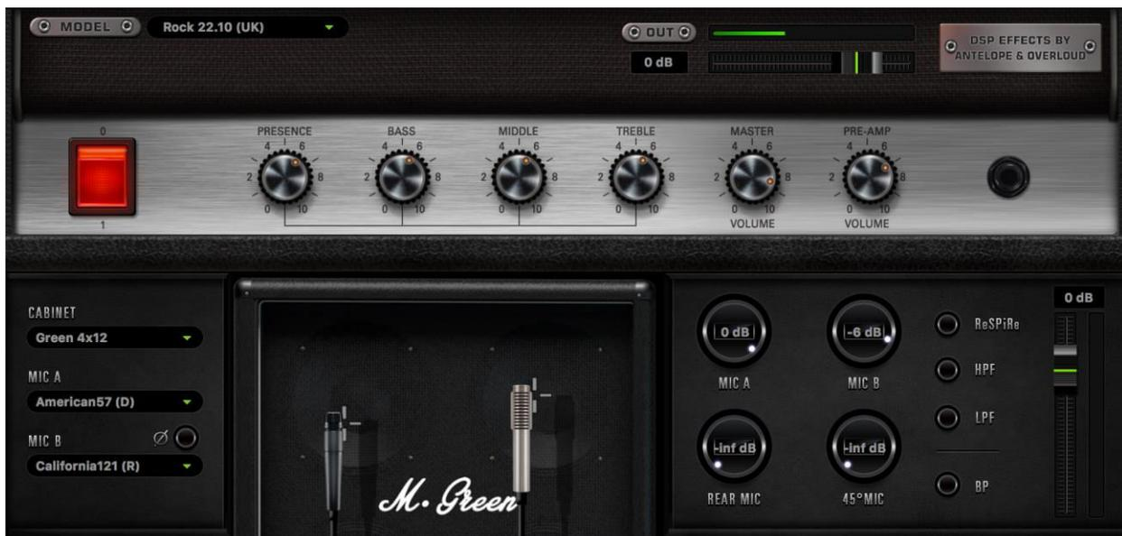
The 80s were marked by a worldwide hard-rock and heavy metal explosion. For amp manufacturers that meant one thing – MORE GAIN. **Rock 22.10** is FPGA-modeled after the amp, which handled this new sound the best. It achieved its savage and aggressive sound by having extra clipping diodes and its EQ was placed after the third gain stage. Antelope's 22.10 features controls for Presence, Bass, Middle and Treble plus Master and Pre-Amp Volume for even more detailed Gain control.
