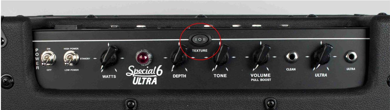
✦ **“Depth” knob is an 11-position knob that affects the low frequencies by creating the same “roll off” effect but in the lower frequency range**
